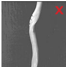
Don't allow the cable to kink, knot, or snag while pulling it off the spool or out of the box; deforming the pair-twist will alter the performance of the cable.
